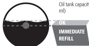
Oil functioning level      Oil refill level
